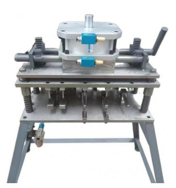
Aluminum window and door pneumatic punching machine Windows processing, and aluminum frame projects such as sun room and pergola. Mainly used for punching various holes or slots, such as keyholes, hinge holes, drain holes, and corner holes.
